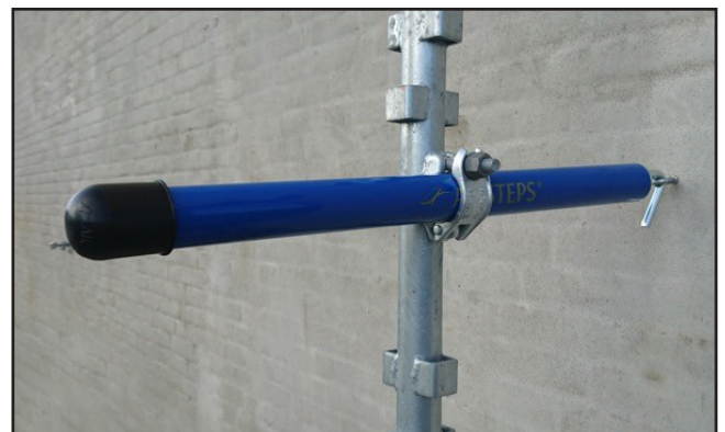
Equipped with a steel hook Airsteps wall anchor can hold a push/pull of 1000 kg. Photo: Nordic Platform.
